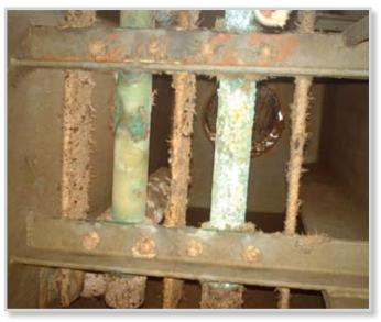
This type of MGPS relies on an external direct current source to be forced into the water from wasting anodes. The anode is in the electrolyte with the sea chest/strainer it intends to protect, and is made more positive than the structure by connecting the DC supply to both the anode and the structure. Cupric lons are produced from the anti-fouling anode, and once fitting will quickly remove existing marine growth and can be used in seawater suctions and open water applications.
